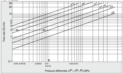
How to read the graph When a water flow of 2 L/min is generated,  $\Delta P$  Approx. 0.013 MPa for a valve with ø3 orifice.
