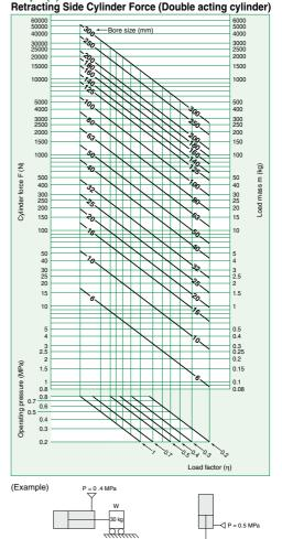
Example 2: To move a load with a 30 kg mass horizontally on a guide as shown in Fig. (2), because the load is the same for both the extending and retracting sides, use Graph (2), which is the retracting side with a smaller force. Determine the load factor of 1, and the operating pressure of 0.4 MPa. Then, seek the point at which it intersects with the load mass of 30 kg, and this will result in a bore size of 40 mm.
