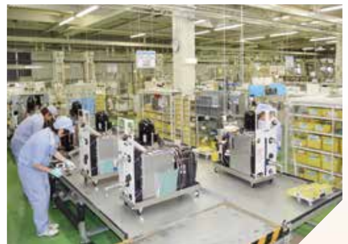
温控器 组装·检查 Temperature Control Equipment Assembly/Inspection
