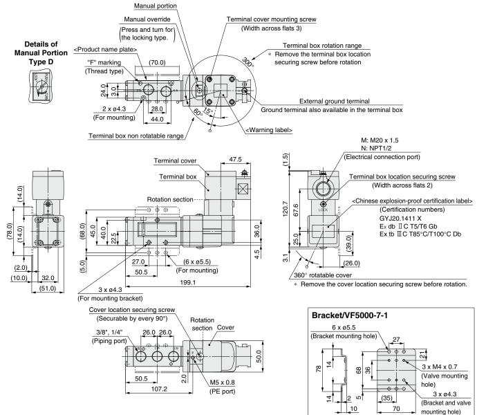
Screw part number: VF5000-17-1(M4 x 37, With spring washer)
