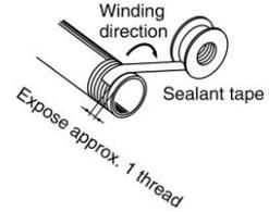
Also, if sealant tape is used, leave 1 thread ridge exposed at the end of the threads.
