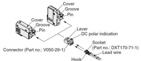
\*In order not to damage the connector and cover, do not pull the lead wire excessively (with a force of 10 N or more).
