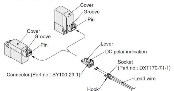
\*In order not to damage the connector and cover, do not pull the lead wire excessively (with a force of 30 N or more).
