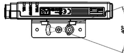
**Mounting angle adjustable range of the L-bracket**
