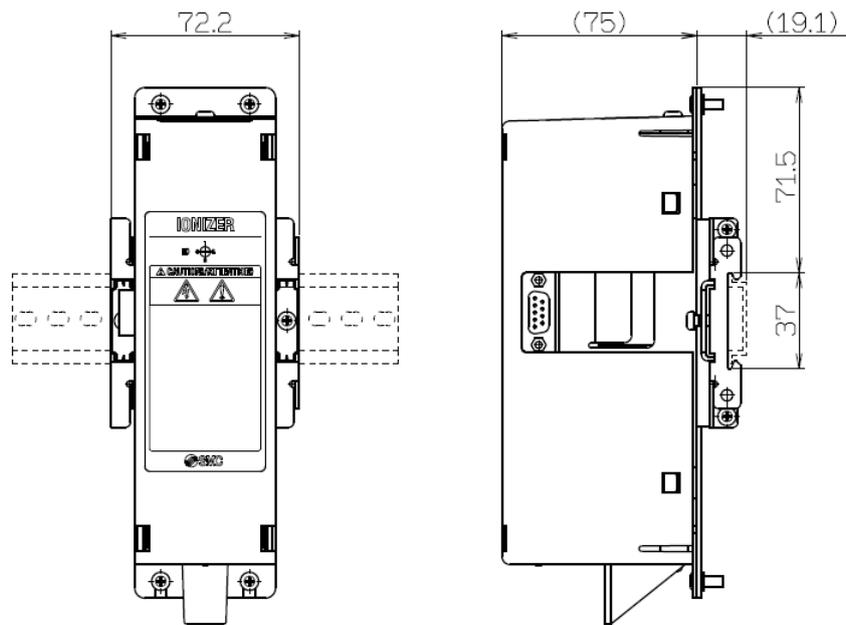
High voltage power supply module IZTP42 (IZT42)
