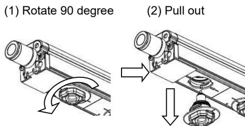
Removal procedure of emitter cartridge
