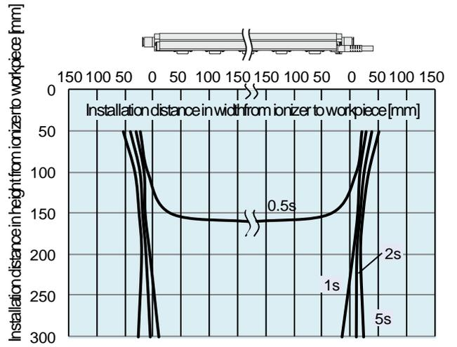
4) With Energy saving high-efficiency cartridge, Supply pressure: 0.3 MPa
