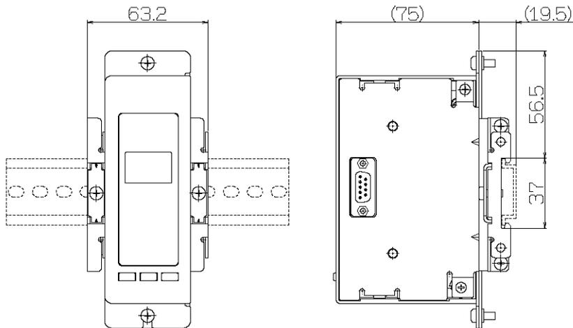
High voltage power supply module IZTP40, IZTP41 (IZT40/41)
