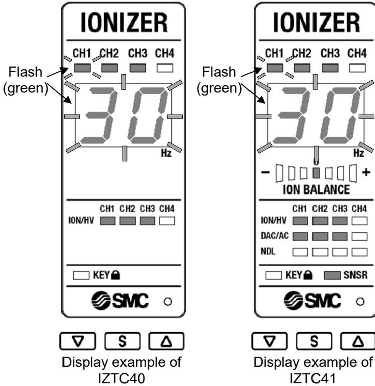
Example of frequency setting mode for CH1.
