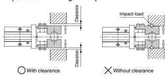
2) Stroke end when gripper is moving
