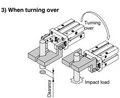
3. Adjust the gripping point so that an excessive force will not be applied to the fingers when inserting a workpiece.
