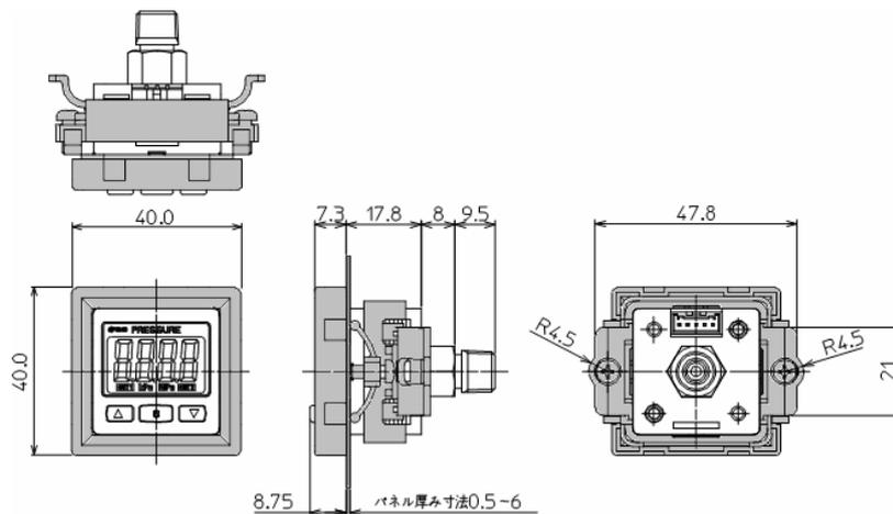
※Panel mount adapter can be rotated by 90 degrees for mounting.
