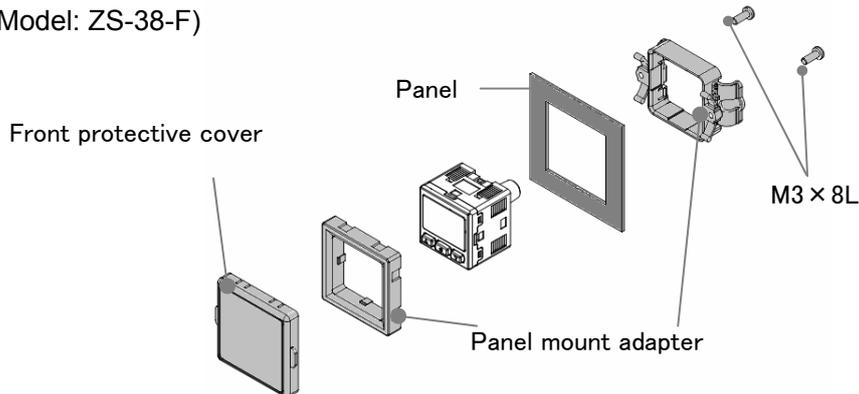
※The panel mount adapter and the front protective cover can be rotated by 90 degrees for mounting.
