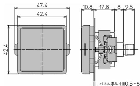
※The panel mount adapter and the front protective cover can be rotated by 90 degrees for mounting.
