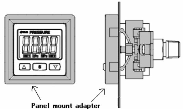
Example) Z/ISE30A can be mounted to a panel that had the Z/ISE40 or Z/ISE4 series mounted.
