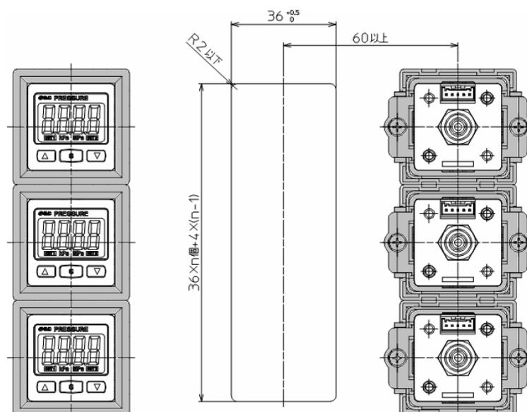
**When ZS-38-F(36 mm<sup>2</sup> square panel mount adapter + 36 mm<sup>2</sup> square front protective cover) is used**
