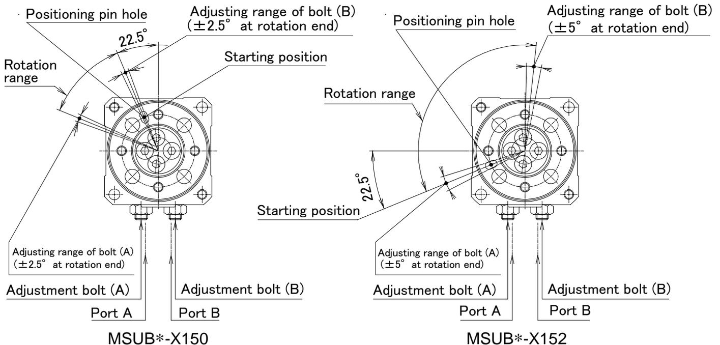
**Feature 1: Rotation angles can be selected in the range of 15° to 165° in increments of 15°.**
