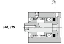
Single acting, spring extend/ with auto switch (built-in magnet)
