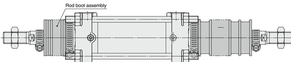
\* Replaceable with the rod boot assembly
