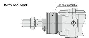
\* Replaceable with the rod boot assembly For details on replacement part numbers, refer to page 248.
