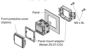
\* The panel mount adapter can be rotated by 90 degrees for mounting.
