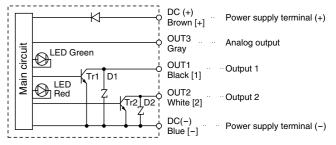
Note) The symbol shown in [ ] means the pin assignment of connector connection type.
