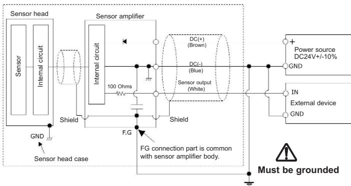
The GND connection must be grounded to an earthing resistance of 100 ohms or less.
