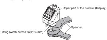
When tightening, do not hold the ISE70/ISE71 body with a spanner.
