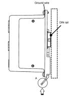
Hook the driver onto the DIN rail and press the lever in the direction of the arrow to lock the driver to the DIN rail
