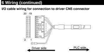
• Parallel I/O wiring for NPN and PNP connection
