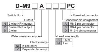
This product is a Solid State Auto Switch of direct mounting specification. Switch should only be used in areas in which potentially explosive atmospheres are unlikely to be present or only present for short periods of time.
