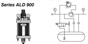
The intended use of the ALD series is to supply lubricating oil to the pneumatic circuit. Lubricant flow is controlled by adjusting the differential pressure in the airline.
