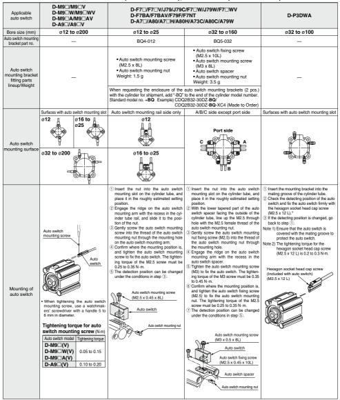
Note) Auto switch mounting bracket and auto switch are enclosed with the cylinder for shipment. For an environment that needs the water resistant auto switch, select the D-M9DA(V) type. Auto switch mounting bracket for the D-F7BA(V) type uses BQ4-012 and BQ5-032 normal specifications (metal screw).
