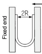
Bend the tube into a U shape at a temperature of 20°C. Fix one end and bend the loop gradually. Measure 2R when the tube breaks or is crushed.
