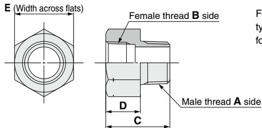
For converting the thread type of an IN/OUT fitting for air dryers.
