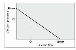
The flow rate characteristics indicate the relationship between the vacuum pressure and the suction flow of the ejector. They also show that when the suction flow changes, the vacuum pressure also changes. In general, this indicates the relationship at the ejector's standard operating pressure.
