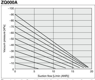
The actual suction flow at the point of suction varies depending on the piping conditions to the vacuum port. (The above graph shows the value when V port is  $\phi$ 6.)
