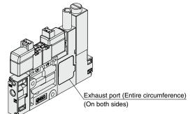
For the port exhaust specification, back pressure may increase depending on the size and length of the piping connected to the exhaust (EXH) port. Ensure that the back pressure does not exceed 0.005 MPa (5 kPa). Do not operate the ejector or apply pressure to the exhaust port with the exhaust port closed. This increases the pressure in the product and can damage the vacuum ejector.
