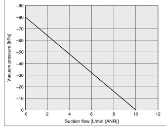
ZQ10 A: Flow Rate Characteristics Supply pressure: 0.43 MPa
