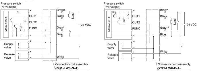
\*1 The gray wire (FUNC) is connected when operating the supply valve by energy saving control (for workpiece adsorption). (For details, please refer to the Operation Manual for the ZQ-ZSVD-D-A series on the SMC website.)
