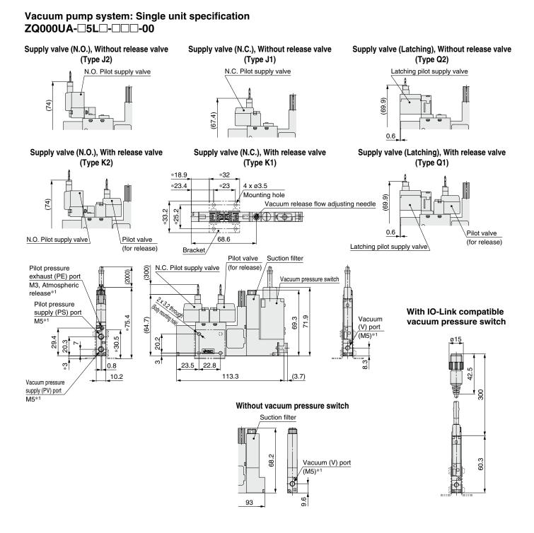
\*1 The pitches of PV, PS, PE, and V ports are determined assuming the use of One-touch fittings.
