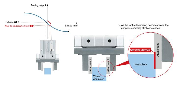
The difference between the measured value and the threshold value can be displayed using the function provided on the display sensor monitor. (Example) When the value at which the master workpiece is gripped is set as the threshold value, the difference can be checked each time.
