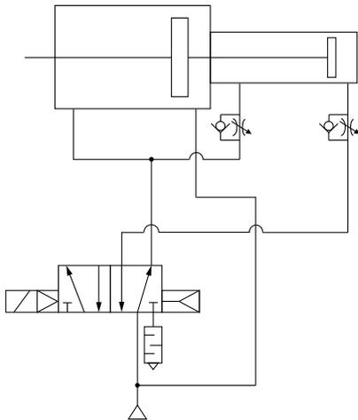
4. Supply the same amount of air pressure to both the assist cylinder and the supply port at all times. If the supply pressure differs, a malfunction may result.
