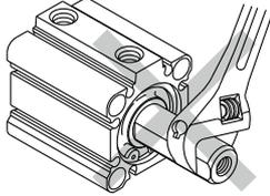
2. Avoid using the air cylinder in such a way that rotational torque would be applied to the piston rod. Failure to do so may result in the loosening of the joint screw part inside the cylinder, leading to unexpected failure.
